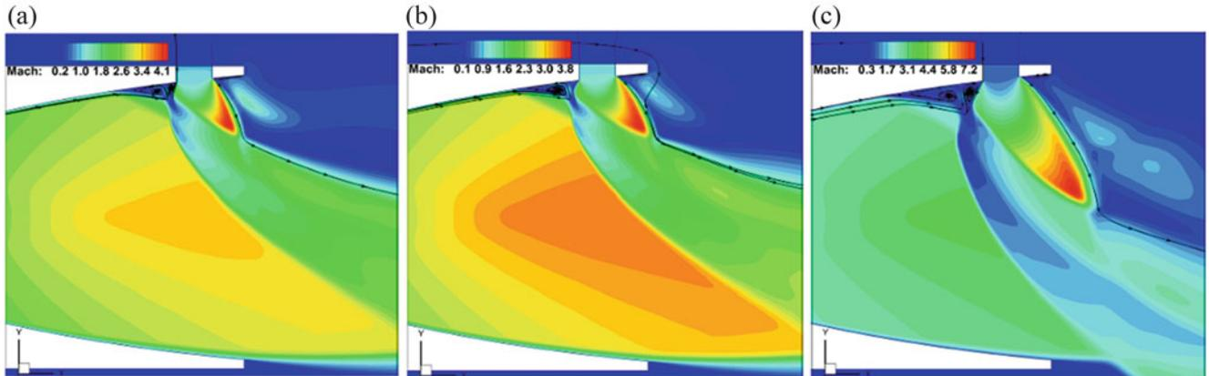
**Fig. 5** Mach contours plots, (a) Ar-Air, (b) CO<sub>2</sub>-Air, (c) He-Air, in symmetry plane of the TIC nozzle at  $f_m = 0.076$
