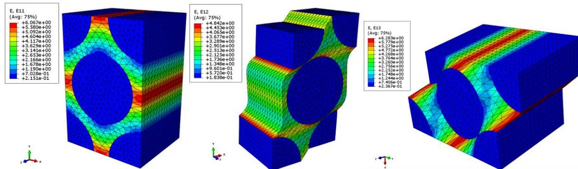
Figure 3 Deformed REV for the microscopic homogenization of yarns with boundary conditions sets: (left) 11, (center) 12 and (right) 13.
