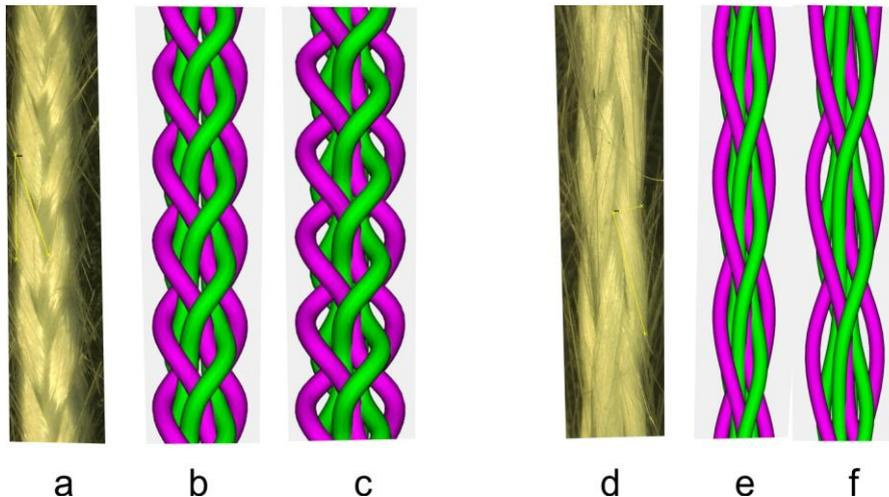
Figure 2 Investigated braids for beams a) and d) produced structures with 9ppc and 4.5ppc, b) and e) - modelled geometry in correct scale, but with small yarn intersection regions, c) and f) slightly expanded geometry, free of intersections
