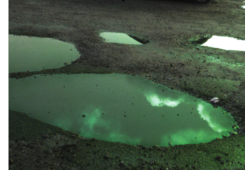
Fig. 2: Illustration of the behaviour of HSL images when the scene has reflective areas. Here, four clearly visible puddles are strongly coloured green (green represents the angle of polarization, corresponding approximately to 90 degrees according to the HSL color wheel [33]).
