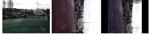
Fig. 4: Experimental validation of augmentation process. Images (a) and (b) are acquisitions with physical rotations applied to the camera. Image (c) is the result of augmentation applied to image (a). Note the correct recovery of angle information.
