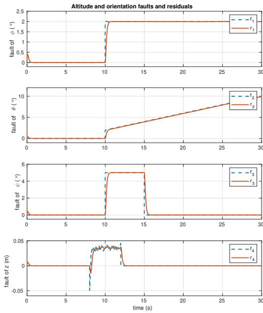
Fig. 4: Faults vs residuals for system states
