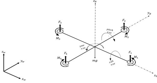
Fig. 1: Quadrotor schematic with motors forces and moments
