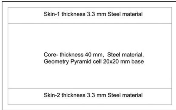
**Figure 1.** Sandwich panel with pyramid lattice core.
