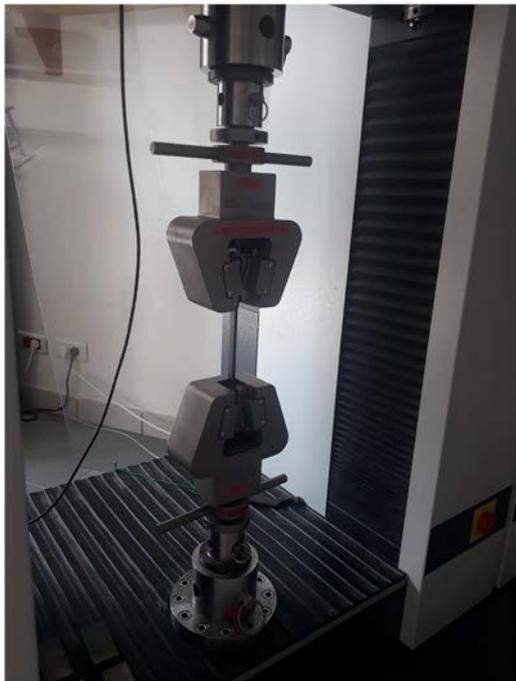
**Figure 4.** The sample under tensile test.
