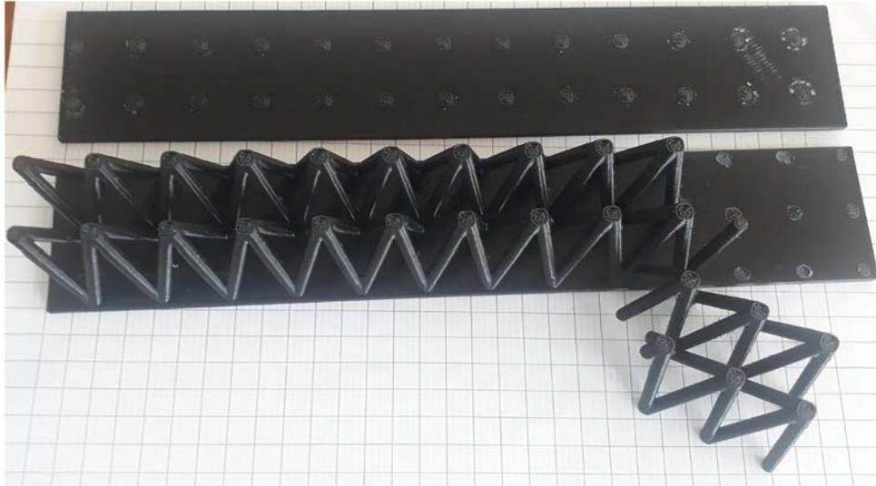
**Figure 8.** Rupture aspect for the pyramid core sandwich panel.
