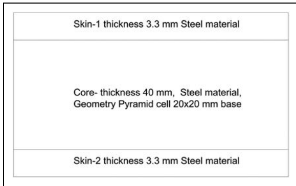
Figure 1. Sandwich panel with pyramid lattice core.
