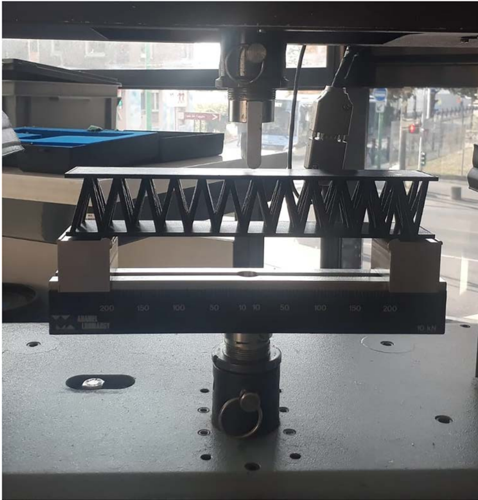
Figure 6. Experimental bending test.
