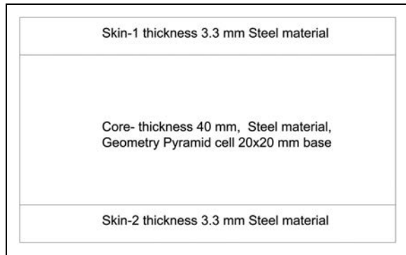
Figure 1. Sandwich panel with pyramid lattice core.
