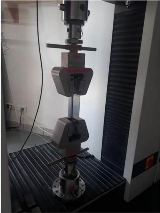
Figure 4. The sample under tensile test.
